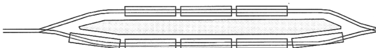
(c) Rapid transit station with simultaneous parallel stopping at an island platform or for bypassing of local by express trains
