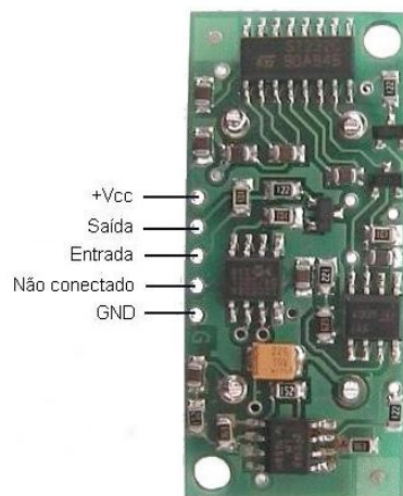
Figura 4 – Pinos do sonar Devantech SRF04
