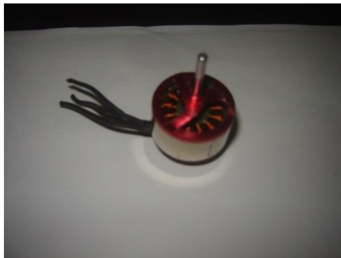
Figura 5 - Motores brushless EMAX CF2822 Electronic Speed Controllers
