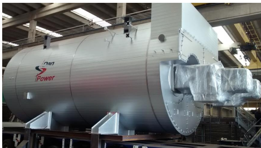
Figura 4 – Caldeira Flamotubular TPS-30000 (DANPOWER, 2021).
