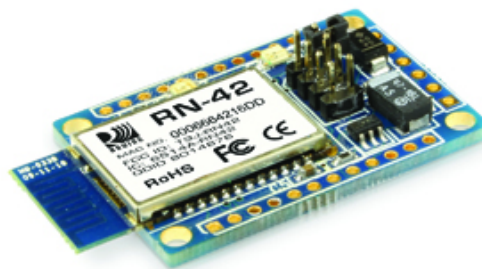
Figura 31: Módulo RN-42-SM [Folha de dados: http://www.rovingnetworks.com/resources/download/20/RN_41_SM_RN_42_SM. ]
