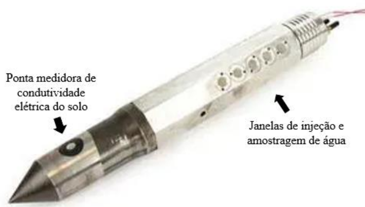
Figura 6 – Sonda Hydraulic Profiling Tool – Groundwater Sampler (HPT- GWS)
