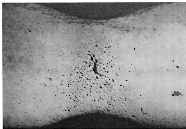
Figure 10. Section through the neck of a tensile specimen of copper. Cavities coalescing in the neck before fracture. Load direction: horizontal. [K.E. Puttick, 1958].
