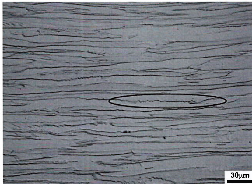
Figure 27. Serrated Interphase Boundaries in the interphase between ferrite and austenite. Load direction: horizontal.
