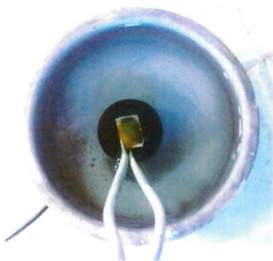
Figure 12. Yellow surface of the polished DSS during attack with oxalic acid. Top view.
