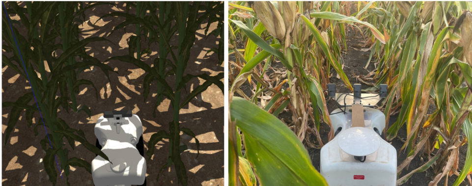
Figure 1: The figure illustrates the Sim2Real transition of the TerraSentia robot. The left shows the TerraSentia in a Gazebo simulation environment [1], while the right depicts the real robot performing the same task in a plantation.
