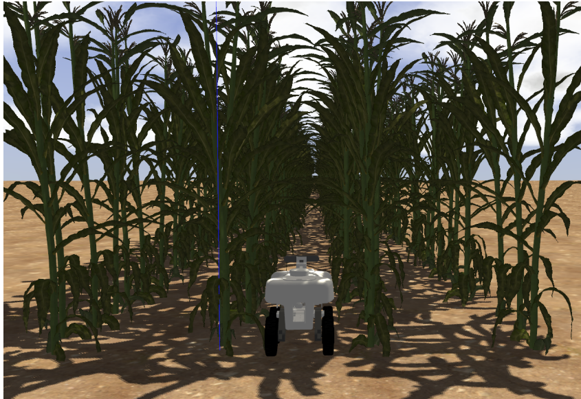
Figure 4: Simulation environment in Gazebo for the crop following task, featuring the TerraSentia Robot. The environment includes four rows of sorghum, spaced 0.7m apart, with the robot positioned to follow the center path. Adjacent rows are included to simulate real-world LiDAR point cloud leakage. The 120m long rows represent fully developed sorghum.
