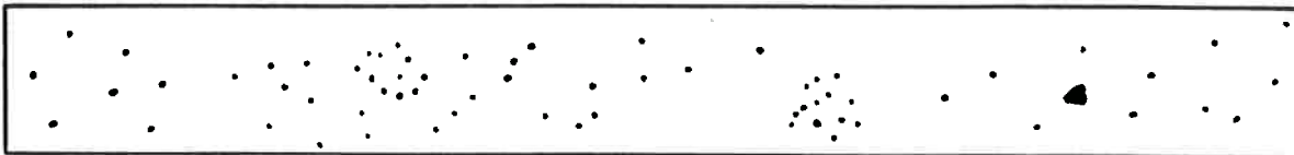
TYPICAL QUANTITY AND SIZE PERMITTED IN 6 IN. LENGTH OF WELD OVER 1/2 IN. TO 1 IN. THICKNESS
