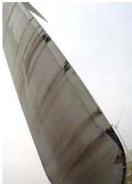
Figura 5.36: Leading edge tape erosion
