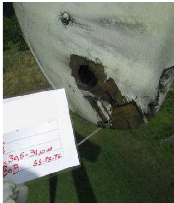
Figura 5.46: Bladetip stroke by lightning
