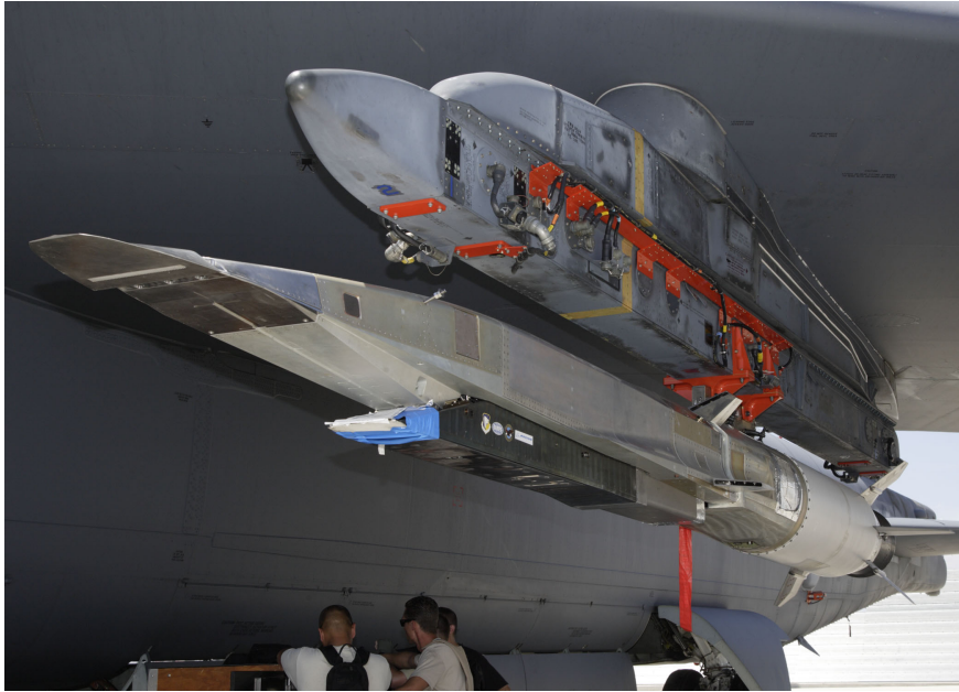
Figure 6 – An X-51, A Waverider hypersonic flight test vehicle is uploaded to an Air Force Flight Test Center B-52 for fit testing at Edwards Air Force Base on July 17, 2009.
