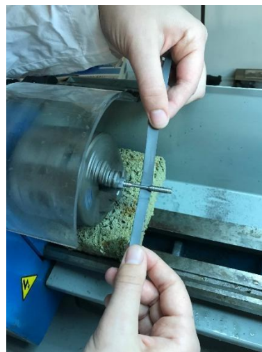
Figure 11 - The polishing process of the samples used in the fatigue tests.
