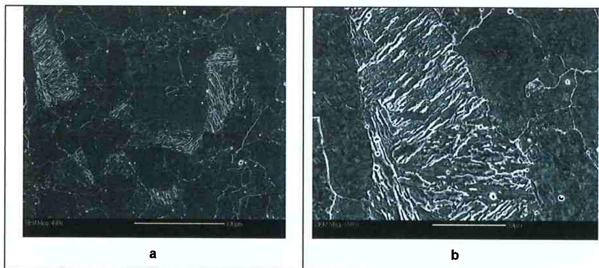
Figure 31 - SEM images of the 0,2 Mo sample treated for 72 hours at 675 °C.
