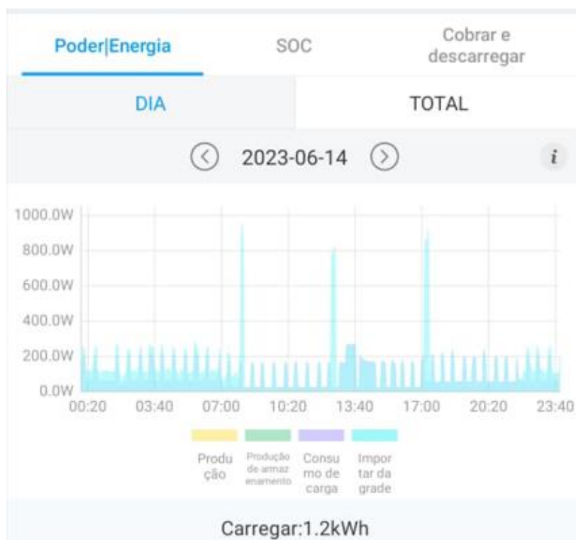
Figura 3.22 - Monitoramento ShinePhone do inversor OFF-GRID Growatt
