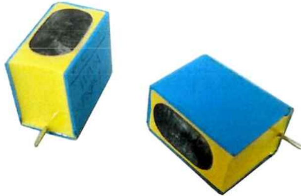
Figure 2.2.: Transversal Cut of Capacitor
