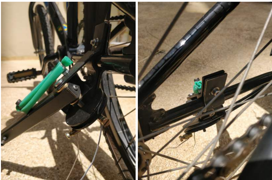
Figure 55 – Close-up view of the support mechanism attached to the bicycle
