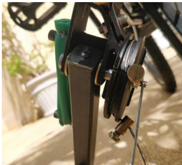
Figure 58 – Close-up view of the support mechanism showing the reel part and cable fastener screws
