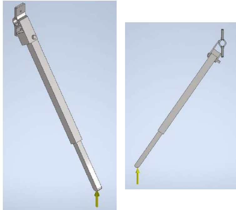
Figure 48 – Direction of force with magnitude 410N applied to support mechanism in finite element method static structural simulation
