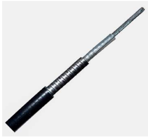
Figure 34 – Cut-away Bowden cable. From left to right: protective plastic coating, helical steel wire, inner sleeve to reduce friction and inner steel cable
