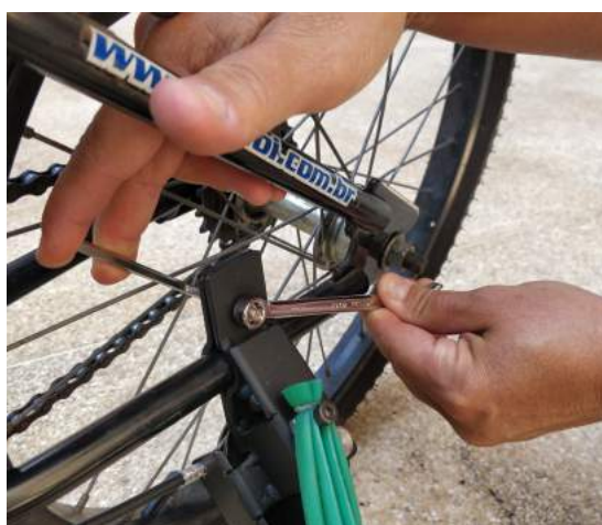
Figure 60 – Steps required to install the prototype to a bicycle From left to right: fasten screws and nuts at the chainstay and fasten screws at the twist throttle
