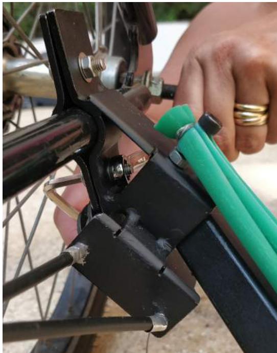
Figure 57 – Close-up view of the support mechanism showing the where cables are connected
