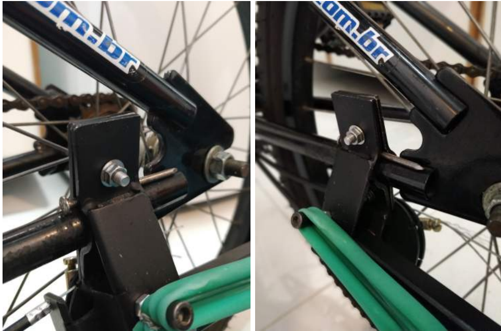
Figure 62 – Adaptation made between test 2 and 3 to prevent rotation of support mechanism
