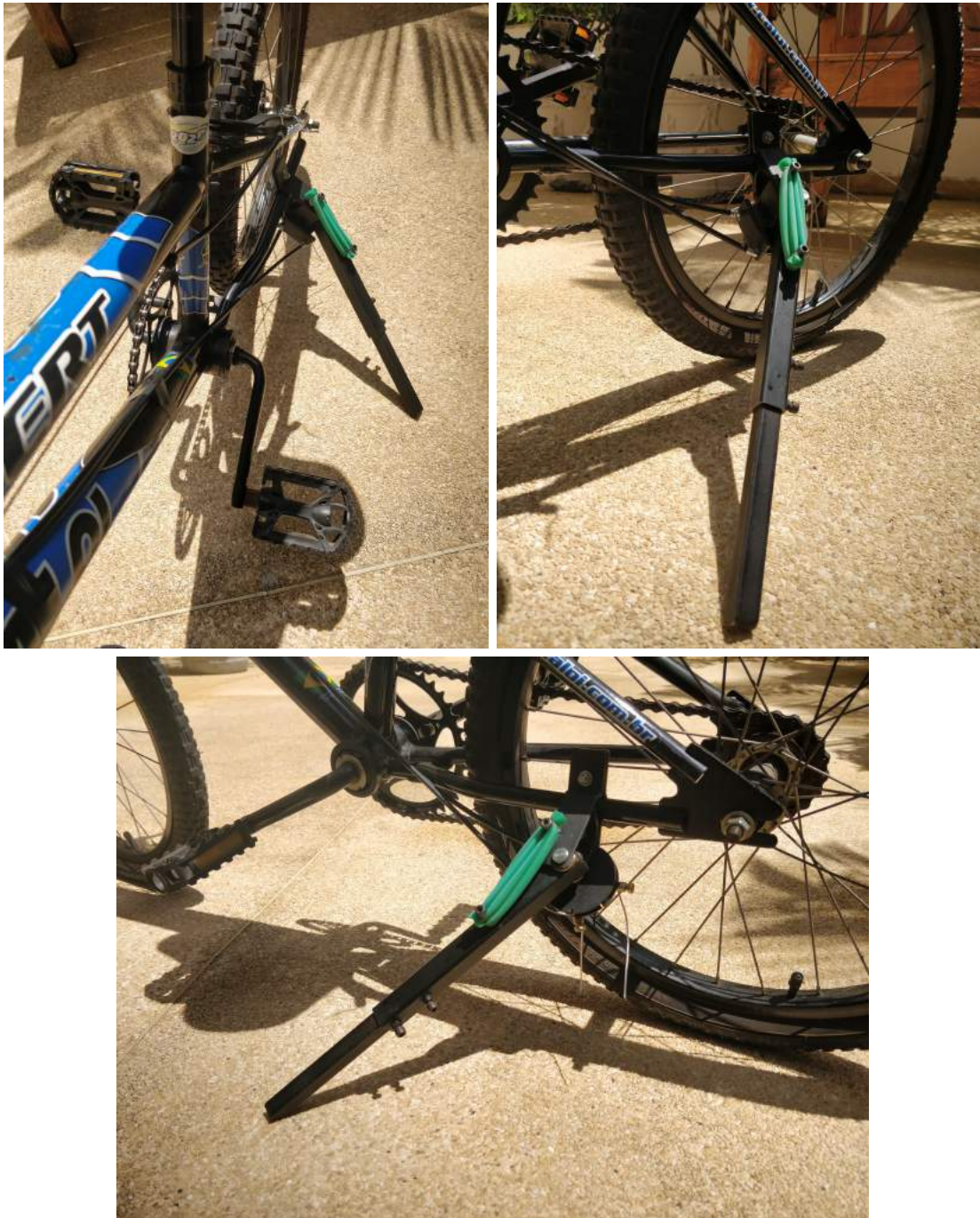
Figure 53 – Close-up view of the deployed support mechanism
