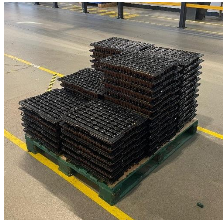
Figure 7: Reusable thermoformed containers used for flask supply
