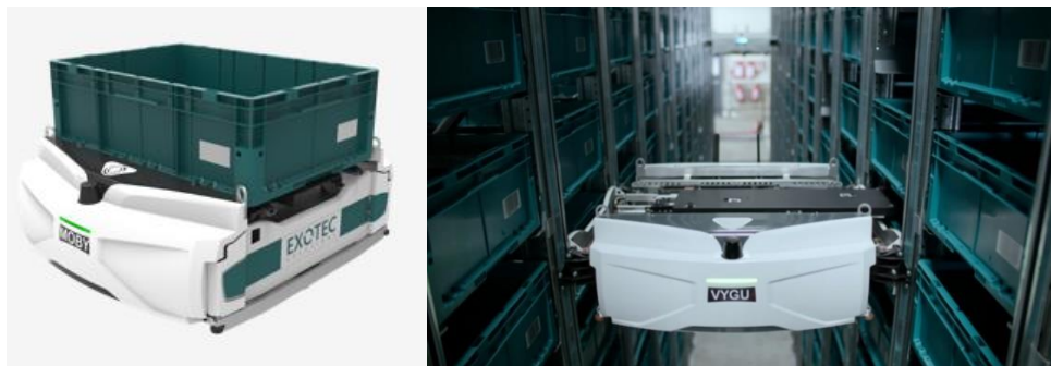
Figure 18: Skypod robot (left) and skypod robot picking a product in a high tier (right)
