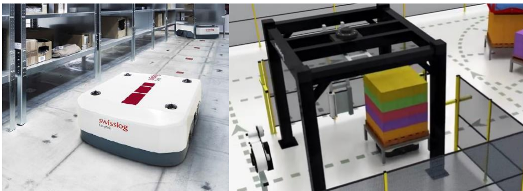
Figure 16: Carry AGV (left) and Carry AGV taking the mixed pallet to the wrapping area (right)
