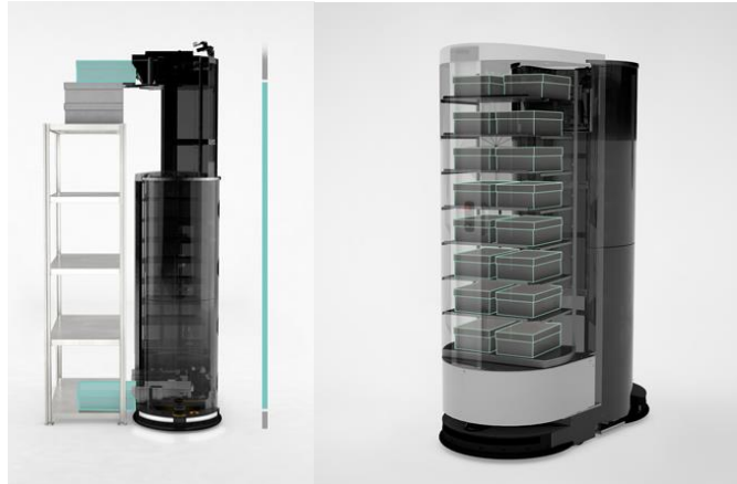
Figure 17: TORU robot picking an item (left) and the robot with the storage filled with products (right)
