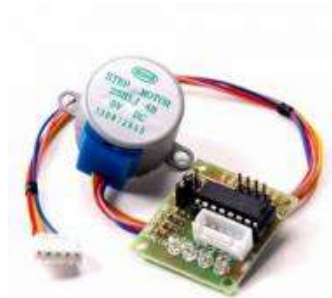
Figura 22 – Motor 28BYJ-48 com driver ULN2003
