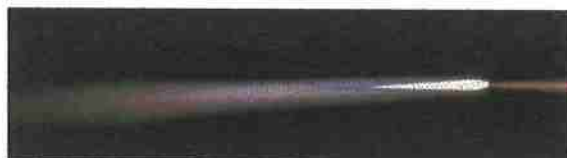
Chama Carburante, T_{\text{máx}} 3.150°C
