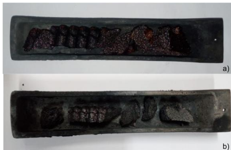
Figure 22: Sample 1, a) before carbonization with argon at 1000 °C, b) after carbonization with argon at 1000 °C.
