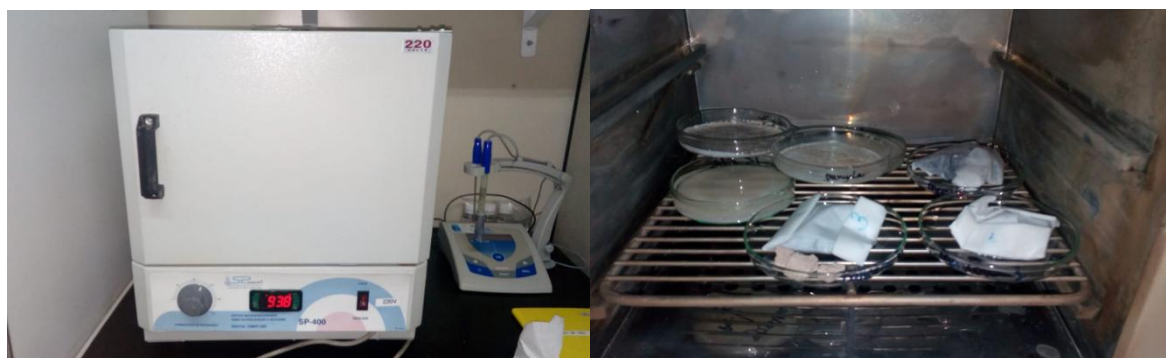
Figure 24: On the left, photograph of the oven used for the drying step. On the right (inside the oven), petri dishes containing the samples wrapped in filter paper.
