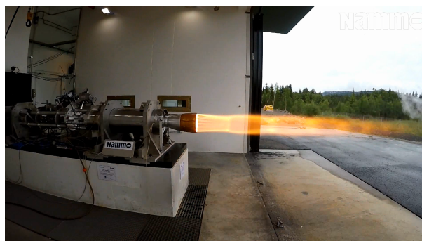
Figure 5 – Hybrid Rocket Nucleus test before launch by (Nammo, 2023)
