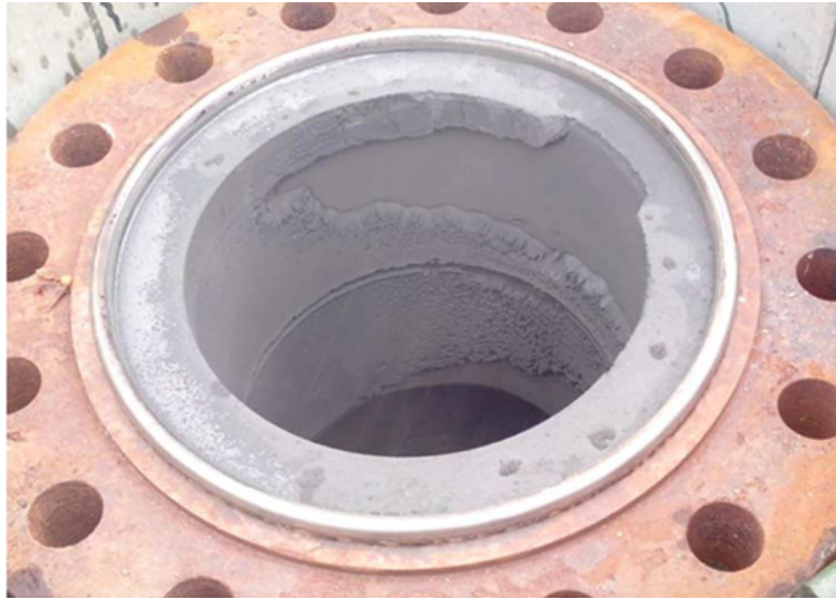
Figure 3: Generalized acid corrosion at the head of a geothermal well [8]
