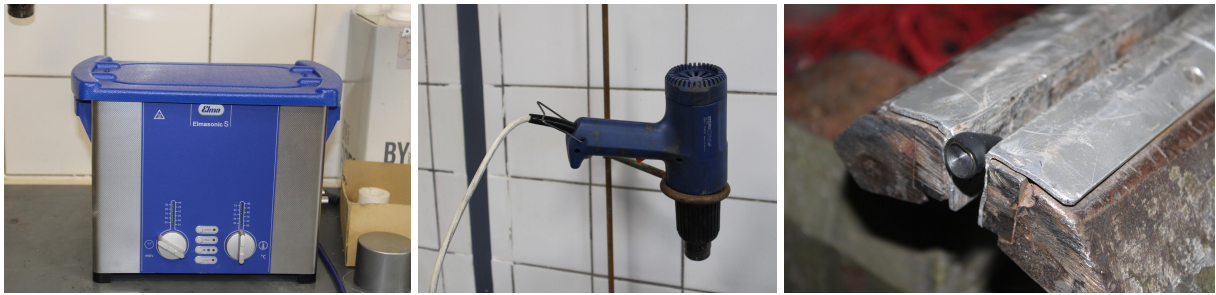
Figure 10: Thermal Ultrasonic Bath (left) | Hot Air Thermal Blower (center) | Heat Shrinkable Tubing application (right)
