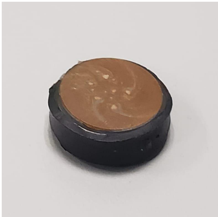
Annexed Figure 8: Carbon Steel Sample clearly corroded after experiment with 10 mg/L TurboDispin 4363
