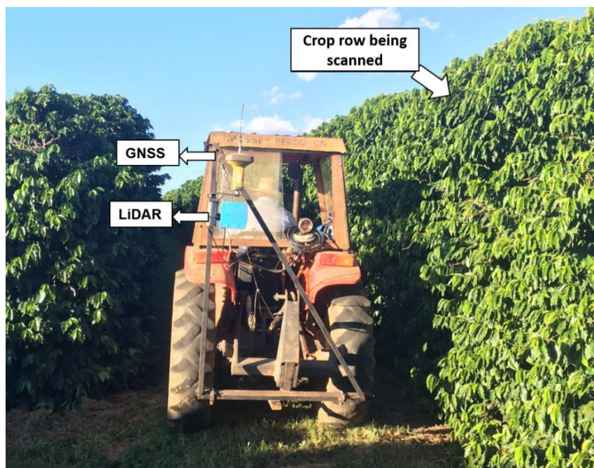
Figure 1. Laser scanner sensor and GNSS on the structure used for the data acquisition (KARP et al., 2018)
