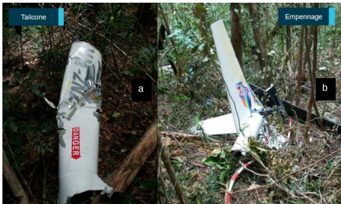
Figura 40 – Destroços de (a) carenagem de rotor de cauda (b) e cauda . Fonte: https://www.atsb.gov.au/publications/investigation_reports/2016/aoir/ao-2016-156/
