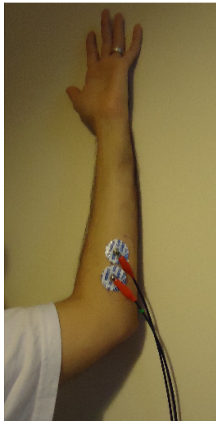
Figure 9 - Electrodes positioning and connection
