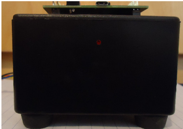
Figure 31 - Device side view with bluetooth LED status indicator (red)
