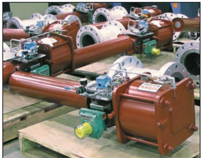
Automated Torqseal® valves destined for a petrochemical facility.
