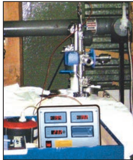
Cold temperature testing to -314°F (-192°C) of the cryogenic Torqseal® valve in our Lyon, France facility.
