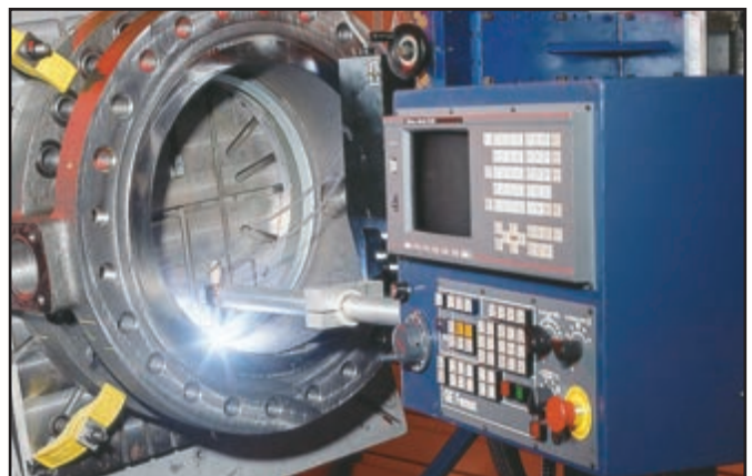
Automated CoCr alloy (cobalt-chrome alloy) deposit system.
