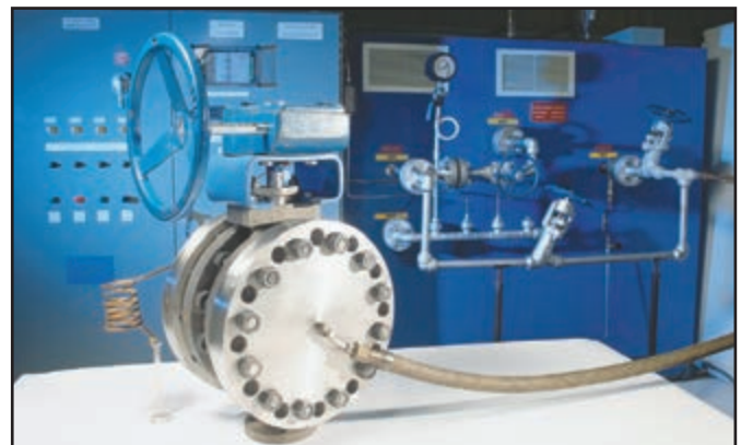
Superheated test on NPS 14 (DN 350) class 150 valve.
