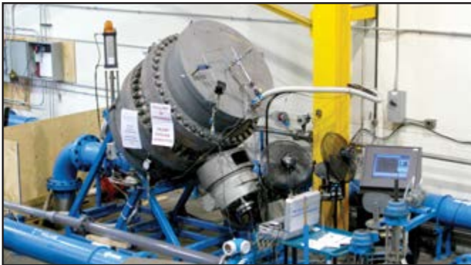
Velan Torqseal® valve with renewable seat ring and TiO_2 plasma sprayed seat surface.
