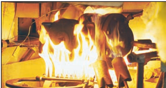
Velan Torqseal® valve being exposed to extreme temperatures of 1800°F (980°C).
