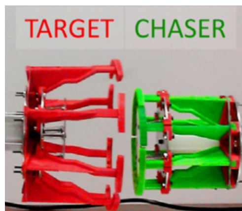
Figure 35 – Semiandrogynous connector in docking process. The chaser one on the left opening up for "grabbing" the target one on the right.
