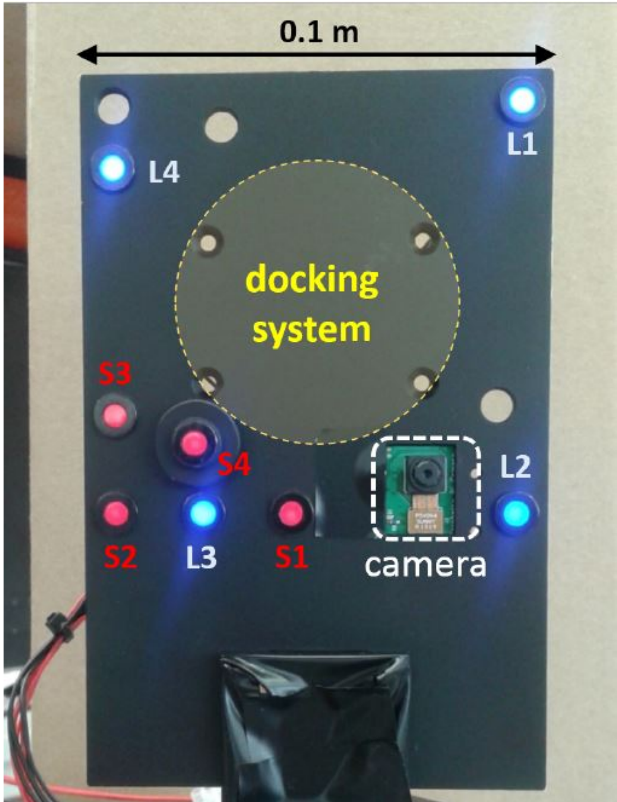
Figure 59 – Padova probe/drogue connector proposed LED fiducial pattern.
