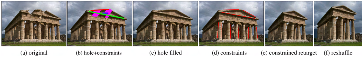
Figure 2.4: PatchMatch structure synthesis. (a) Original image. (b) User marks a hole (magenta) and line constraints (red/green/blue) to elucidate the continuity of the roofline; (c) The hole is filled in. (d) User inputs line constraints for retargeting, (e) which eliminates two columns automatically. (f) Reshuffling: user translates the roof upward. Source: Barnes et al. [13]
