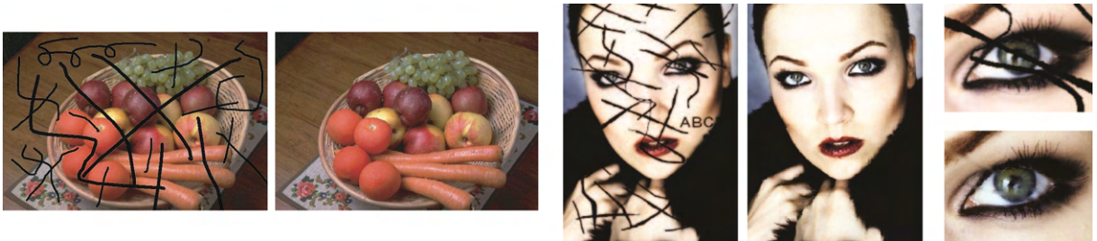
Figure 2.6: Inpainting results with the proposed FMM-based method. On the right, a close-up of the inpainted eye is presented. Source: Telea [14]
