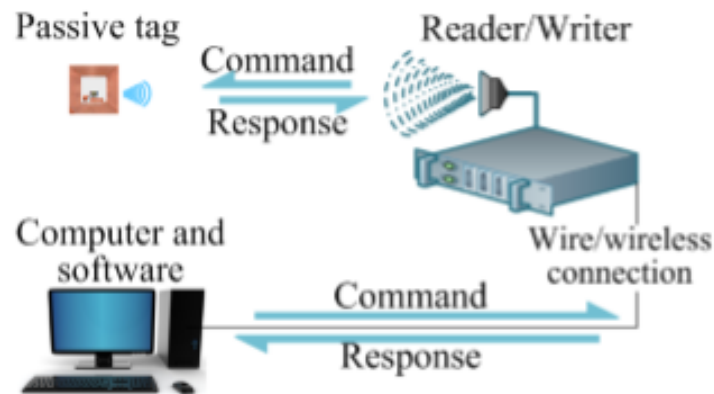
Figure 4: Representation of a Passive RFID system (extracted from [34]).
