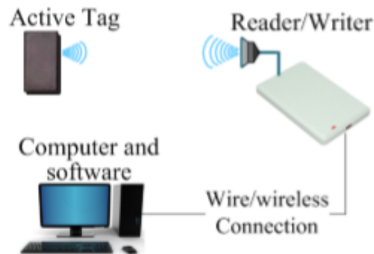
Figure 5: Representation of an Active RFID system (extracted from [34]).
